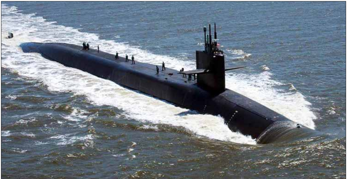
Ohio-class guided missile submarine USS Florida (SSGN-728). Florida was the second of four SSBN submarines to be converted to the guided missile SSGN platform. (Photo credit: Photographer's Mate 2nd Class Lynn Friant / U.S. Navy.)
